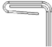
Note: In cases where there is vertical separation between the male and female panel legs crimping to 90° periodically along the seam may be necessary before running the electric seamer.
