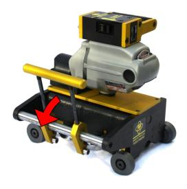
This is a BI-DIRECTIONAL Roof Seamer. Therefore, you may simply place the seamer on the next seam and, after hand crimping, run the machine in the opposite direction of travel. It is important to remember to use extreme caution when reaching the edge of the roof. Stop and disengage the locking handle of the seamer while the wheels remain on the roof panel.
